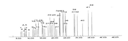
This chromatogram represents a general set of testing conditions chosen for product acceptance. For optimal results in your lab, conditions should be adjusted for your specific instrument, method, and application.
