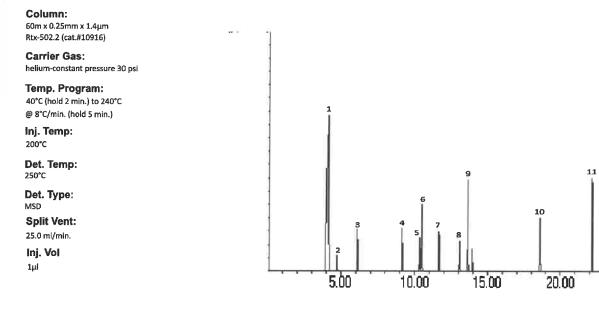
This chromatogram represents a general set of testing conditions chosen for product acceptance. For optimal results in your lab, conditions should be adjusted for your specific instrument, method, and application.
