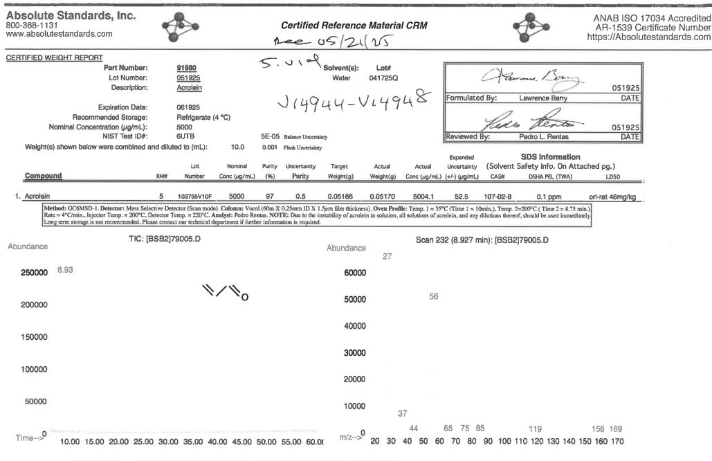
• Standards are prepared gravimetrically using balances that are calibrated by an ISO 17025 certified organization with weights traceable through NIST to the SI kilogram (see above).
