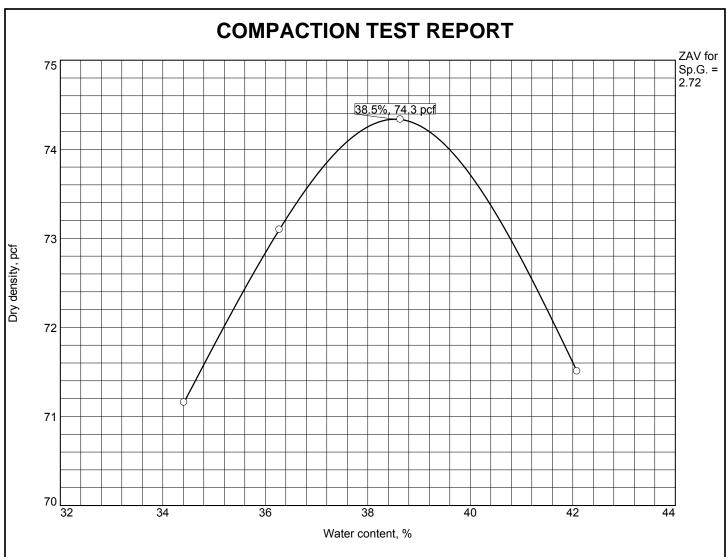
Test specification: ASTM D 698-12 Method B Standard
