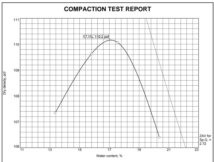
Test specification: ASTM D 698-12 Method B Standard ASTM D4718-15 Oversize Corr. Applied to Each Test Point
